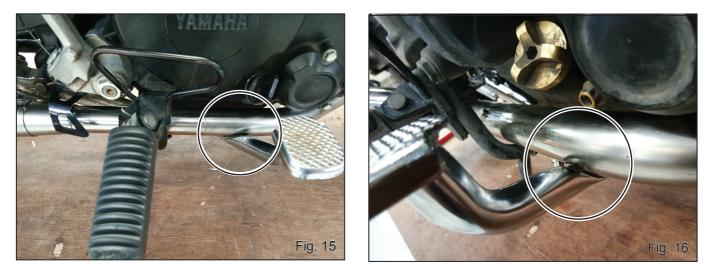
Please Bending Brake Pedal (Bending by Hand) for make gap same picture (See Fig. 17 & 18)
